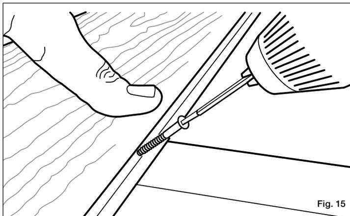
**Step 6** Install a Stowaway hidden fastener clip over the screw and centered over the joist. Fasten using preset screw at a 90° angle through the Stowaway hidden fastener and drive flush with the clip (Fig. 16). The fastener wings must remain level with the joist for the next board to fit correctly (Fig. 17).
