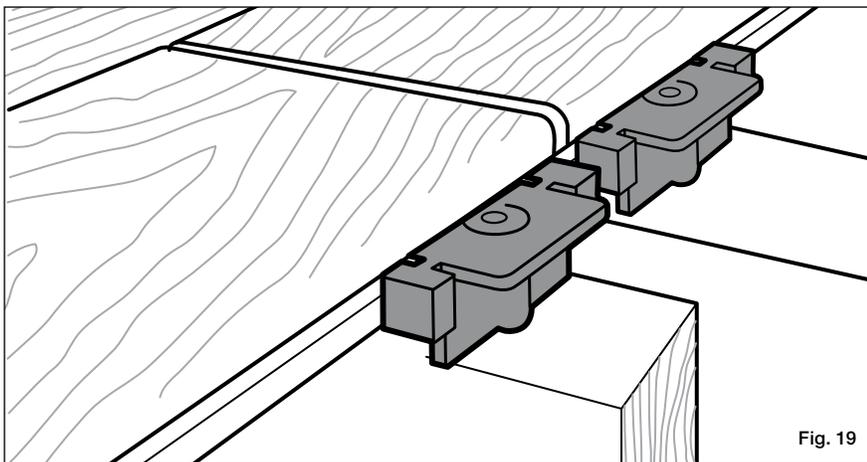
**Step 8** Repeat the process for each board until the outside edge of the final board is fastened with screws. Use fascia to conceal the board profile and inhibit board movement over time. Please refer to the fascia installation instructions for the approved fastening methods for fascia boards.
