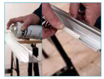
Insert seals, without stretching, on both sides of the bar base. Using silicone lubricant can make installation easier.
