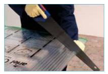
If you need to size the polycarbonate sheets to suit the structure, Corotherm can be easily cut to size and will not crack or shatter.
