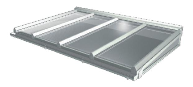
The Ariel Self-Support Roofing System free-spans up to a 4M rafter length, and accommodates 16mm, 25mm and 35mm Corotherm Multiwall Polycarbonate Roofing Sheets. It is not a cantilever design, it requires support at the wall, provided by the Wall Bar, and support at each corner, provided either by Goal Post Legs, or by your own supports. The Self-Support Roofing System can also fix directly into the top of double glazed windows. It is easy to install and low maintenance.
