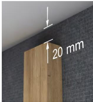
All battens should be level. Any irregularities within the main substrate can mirror through the finished application, potentially leaving a bowed look within a long
