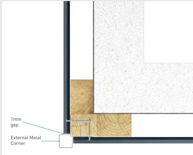
When installing the 2-Part VL Corner Profile below, screw the inner section over the cladding, with the Hardie™ Plank screw, and then click the outer section
