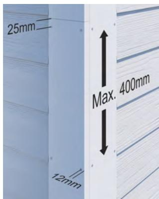
If you do not have access to a brad nail gun, the Hardie® NT3® Trim profile can be installed with stainless steel screws. The screw size should be 3.5 mm × 50 mm with a countersunk head. Pre-drill the Hardie® NT3® Trim profile with a 3.5 mm masonry bit and countersink the hole. Install the screws 25 mm down from the top edges and then in every 400 mm down the length of the trim. The screws
