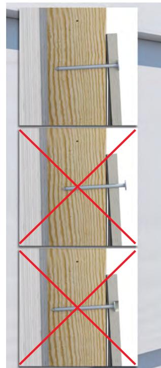
Fix the weatherboard to the vertical timber battens with one nail or screw on **every** batten. The centre line of the nail or screw should be 20–25 mm below the top edge of the weatherboard. When fixing the ends of the cladding ensure the fixing is placed 15 mm in from the edge.
