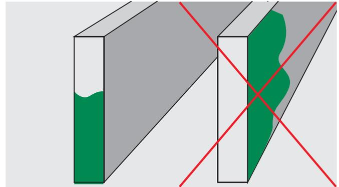
Along with cut edges, Hardie™ Seal edge coating will need to be applied to any exposed back edges of the boards. This is common when using Hardie® Plank weatherboard on edge into window/door reveals.
