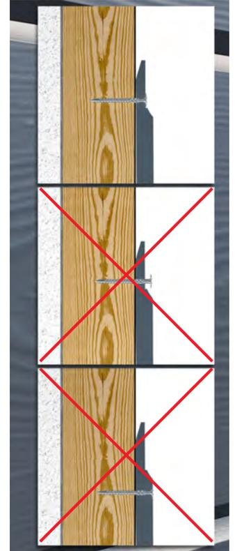
Fix through the tongue part of the weatherboard 25 mm down from the top edge. When fixing the ends of the cladding, ensure the fixing is placed 15 mm in from the edge.
