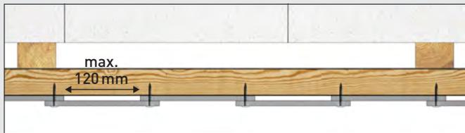
Use the Hardie® Plank weatherboard as a fillet piece to breach gap at bottom and top. Second fix pin these into position.
